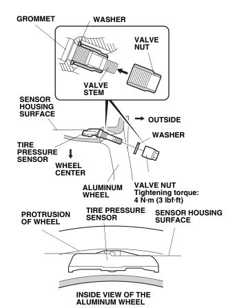
Install the tire pressure sensor:
